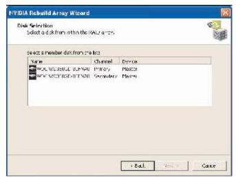
E. Select the drive that you want to rebuild by clicking it from the list, then click Next. The Completing the NVIDIA Rebuild Array page appears.
